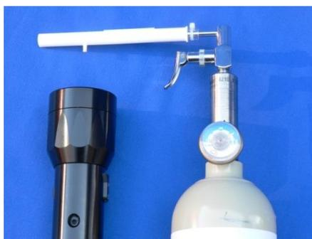
4. Press the Calibration Connector Tube nipple into the inlet port of the PAS V and hold tightly in place.
