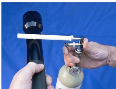
6. Immediately, AND WHILE THE GAS IS STILL FLOWING, press and release the Sensor Control Button which will draw a sample of gas into the unit.
