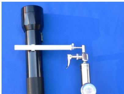
5. Hold the PAS V with your thumb near the Sensor Control Button and press the regulator button so the gas begins flowing.
