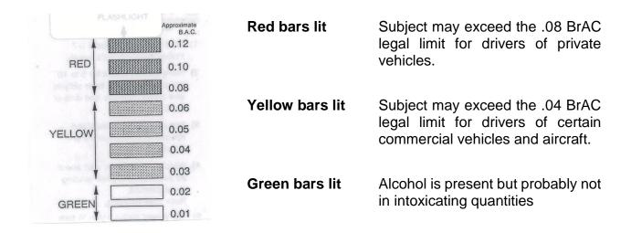
If the PAS Vr. is used according to the manufacturer's instructions in the *active or direct* testing mode, the numeric value indicated on the bar-graph display will give you an accurate verification of the subject's deep lung breath alcohol concentration (BrAC). Results are expressed in terms of weight of alcohol (gm) per volume of breath (liters).
