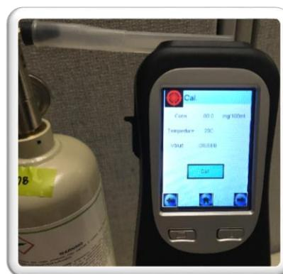
8. Press the gas regulator button, allowing gas to flow into the mouthpiece for 8-10 seconds. While still pressing on the gas, press the **Cal.** button to acquire a sample.
